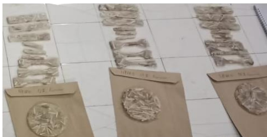
Fig. 2. Representative samples of de-molded fabricated composite samples before trimming
